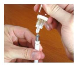
Drip 2 drops directly onto the atomizer wick
