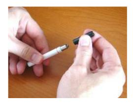
Remove the cartridge from the atomizer
